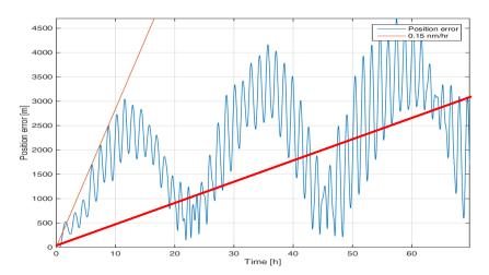
The figure shows such long time behavior of a free inertial navigation (example: data obtained from iNAT-RQT over more than 3 days): <u>Link</u>
