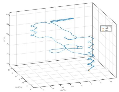
The Plot shows the walk of a firefighter within a builduing: Distance 338 m, final position error 0.5 m
