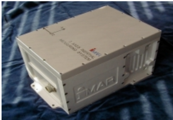
Fig.4: Navigation System iNAV-RQH-N with gyro drift down to 0.002 deg/hr (iMAR, Germany)
