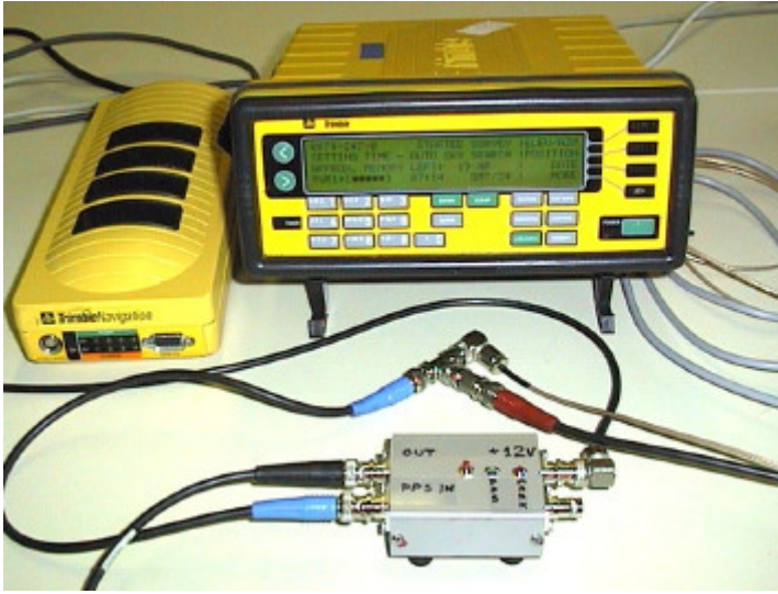
Fig. 4 View of the hardware for the analog time signals (in the laboratory experimentation phase, connected to a Trimble GPS receiver)
